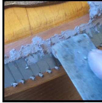
Split-out holes are filled.
